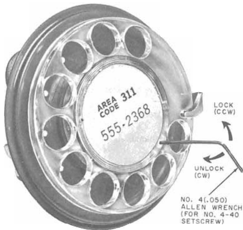
Fig. 7—Installing Fingerwheel on 8U Dial
