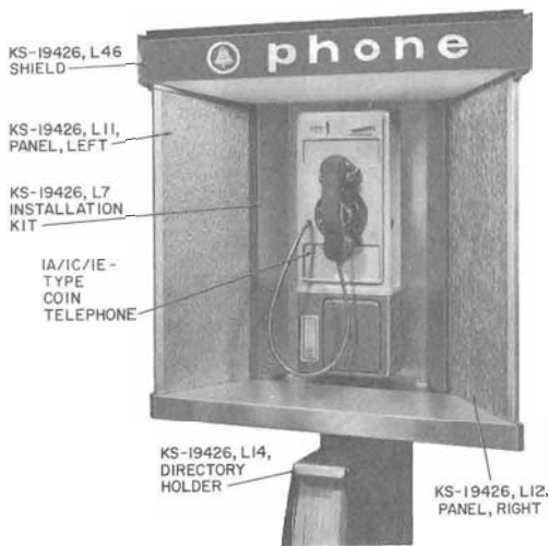
Fig. 10—KS-19426 Mounting Using 1-Type Coin Telephone Set
