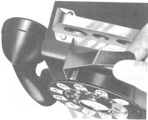
Fig. 29—Method For Installing P-14A544 Coin Deflector
